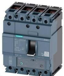
CIRCUIT BREAKER 3VA1 IEC FRAME 160 BREAKING CAPACITY CLASS N ICU=25KA @ 415 V 4-POLE, LINE PROTECTION TM240, ATAM, IN=160A OVERLOAD PROTECTION IR=112A ...160A SHORT CIRCUIT PROTECTION II=5...10 X IN NEUTRAL PROTECTION 100% BUSBAR CONNECTION
