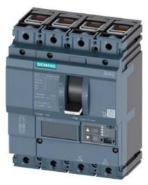
CIRCUIT BREAKER 3VA2 IEC FRAME 100 BREAKING CAPACITY CLASS M ICU=55KA @ 415 V 4POLE, LINE PROTECTION ETU550, LSI, IN=25A OVERLOAD PROTECTION IR=10A ...25A SHORT CIRCUIT PROTECTION ISD=0,6..10X IN, II=1,5..12X IN NEUTRAL PROTECTION ADJUSTABLE (OFF, UPTO 160%) CABLE CONNECTION
