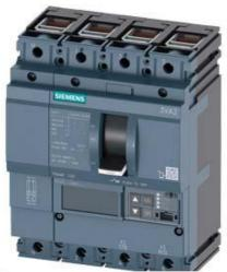
CIRCUIT BREAKER 3VA2 IEC FRAME 100 BREAKING CAPACITY CLASS L ICU=150KA @ 415 V 4POLE, LINE PROTECTION ETU560, LSIG, IN=25A OVERLOAD PROTECTION IR=10A ...25A SHORT CIRCUIT PROTECTION ISD=0,6..10X IN, II=1,5..12X IN NEUTRAL PROTECTION ADJUSTABLE (OFF, UPTO 160%) GROUNDFAULT, SWITCHABLE IG=0,2... 1 X IN, TG=0,050,8MS CABLE CONNECTION
