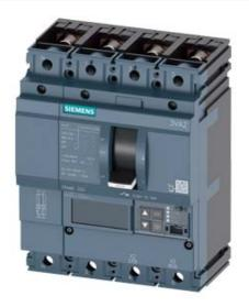
CIRCUIT BREAKER 3VA2 IEC FRAME 250 BREAKING CAPACITY CLASS M ICU=55KA @ 415 V 4POLE, LINE PROTECTION ETU860, LSIG, IN=250A OVERLOAD PROTECTION IR=100A ...250A SHORT CIRCUIT PROTECTION ISD=0,6..10X IN, II=1,5..10X IN NEUTRAL PROTECTION ADJUSTABLE (OFF, UPTO 100%) GROUNDFAULT, SWITCHABLE IG=0,2... 1 X IN, TG=0,050,8MS BUSBAR CONNECTION
