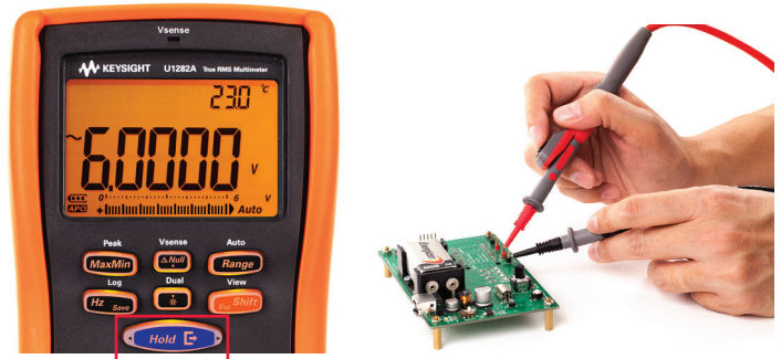
Figure 5. Hold & Export button—one press for three actions: Measure, save it into handheld DMM's memory and send the measurement out via infrared port. Optional U5404A remote switch probe emulates 'Hold & Export' button.
