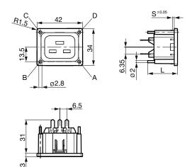
L = Light Pipe Length S = Panel Thickness
