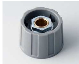
A2523068 RUNDKNOPF 23, ohne Strich ABS (UL 94 HB) staubgrau RAL 7037 23x15mm 6mm
