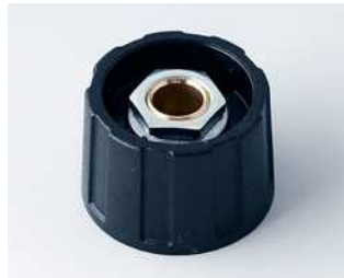
A2523060 RUNDKNOPF 23, ohne Strich ABS (UL 94 HB) schwarz RAL 9005 23x15mm 6mm
