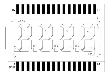
UNLESS OTHERWISE SPECIFIED DIMENSIONS ARE IN MM TOLERANCES: ±0.2MM
