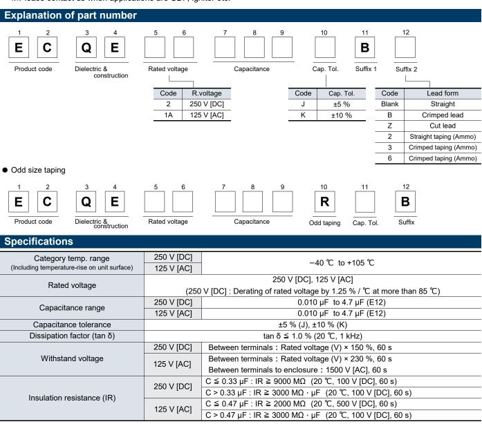
\* In case of applying voltage in alternating current (50 Hz or 60 Hz sine wave) to a capacitor with DC rated voltage, please refer to the page of "Permissible voltage (R.M.S) in alternating current corresponding to DC rated voltage".
