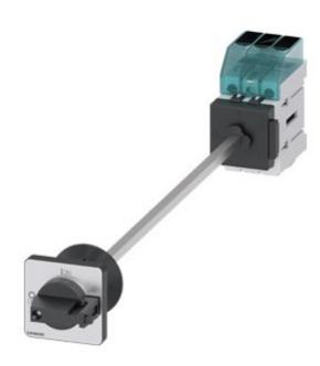
Switch disconnector 3LD3, main switch 3-polig, lu 16A operational switch at AC-23 A at 400 V 7,5 kW floor mounting Base mounting with door coupling center-hole 22,5 mm knob-operated mechanism black  $48 \times 48 \text{ mm}$
