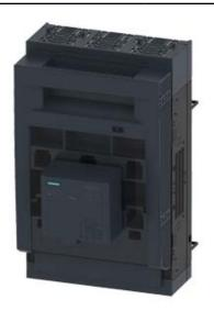
FUSE-SWITCH-DISCONNECTOR 3-POLE, NH1, 250A 60MM BUSBAR SYSTEM COVER LEVEL 32/70 MM FLAT CONNECTOR FUSE MONITORING ELECTRONIC, EFM 10
