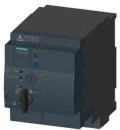
SIRIUS, COMPACT STARTER, REVERSING STARTER 400 V, 110 ... 240 V AC/DC, 50 ... 60 HZ, 8 ... 32 A, IP20, MAIN CIRCUIT CONNECTION: PLUG-IN, W/O TERMINALS, AUXILIARY CIRCUIT CONNECTION: PLUG-IN, W/O TERMINALS
