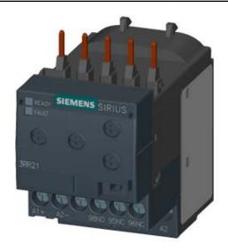
MONITORING RELAY ATTACHABLE TO CONTACTOR 3RT2. SIZE S00 BASIC, ANALOG ADJUSTABLE APPARENT CURRENT MONITORING 1.6 - 16A, 50-60 HZ, 2-PHASE SUPPLY 24 V AC/DC 1 CO CONTACT MONITORING FOR CURRENT OVERSHOOT/UNDERSHOOT PHASE FAILURE, WIRE BREAK WITH OR W/O ERROR LOG ON-DELAY 0-60 S SPURIOUS PEAK SUPPR.0-30 S SWITCHING HYSTERESIS 6% SCREW CONNECTION
