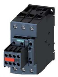
CONTACTOR,AC3:37KW/400V, 2NO+2NC, 230V AC 50/60HZ, WITH PLUGGED-IN VARISTOR, 3-POLE, SIZE S2, SCREW TERMINAL, AUXILIARY CONTACT INSEPARABLE
