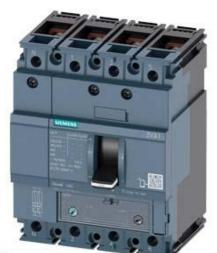
CIRCUIT BREAKER 3VA1 IEC FRAME 160 BREAKING CAPACITY CLASS S ICU=36KA @ 415 V 4-POLE, LINE PROTECTION TM240, ATAM, IN=160A OVERLOAD PROTECTION IR=112A ...160A SHORT CIRCUIT PROTECTION II=5...10 X IN NEUTRAL PROTECTION 100% BUSBAR CONNECTION
