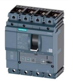
CIRCUIT BREAKER 3VA2 IEC FRAME 160 BREAKING CAPACITY CLASS M ICU=55KA @ 415 V 4POLE, LINE PROTECTION ETU320, LI, IN=63A OVERLOAD PROTECTION IR=25A ...63A SHORT CIRCUIT PROTECTION II=12 X IN NEUTRAL PROTECTION ADJUSTABLE(OFF,100%) BUSBAR CONNECTION
