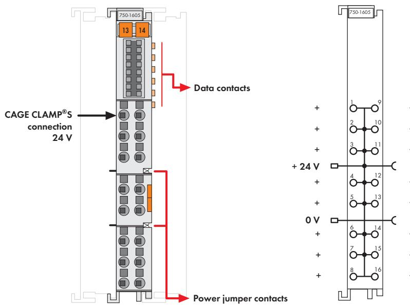
The field side connection module provides 24V power for the inputs of the 16-channel input modules 750-1405 and 750-1406 (also suitable for 8 channel input modules in 1-wire connection), eliminating external terminal blocks.
