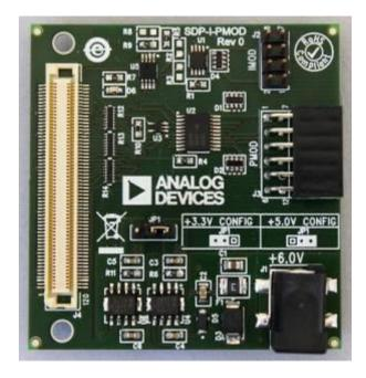
Pictured above is the SDP-I-PMD interposer board which was developed to quickly and easily connect ADI PMOD boards to our system demonstration platform (SDP).
