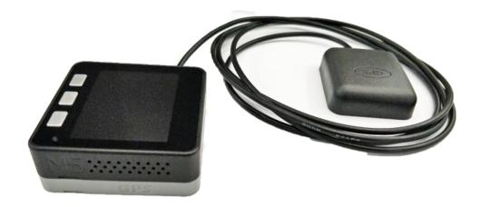
The NEO-M8N integrates a 72-channel u-blox M8 GNSS engine that supports multiple GNSS systems (Beidou, Galileo, GLONASS, GPS / QZSS) and able to receive 3 GNSS systems simultaneously.
