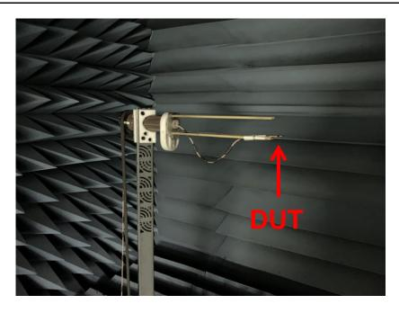
FIGURE4.1.2 ANTENNA LOADED WITH REFERENCE PCB TESTED IN OTA CHAMBER
