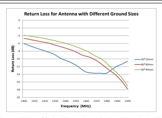
FIGURE 7.4.1 RETURN LOSS OF ANTENNA AT 2.4GHZ WITH DIFFERENT GROUND SIZES FOR CONFIGURE 1
