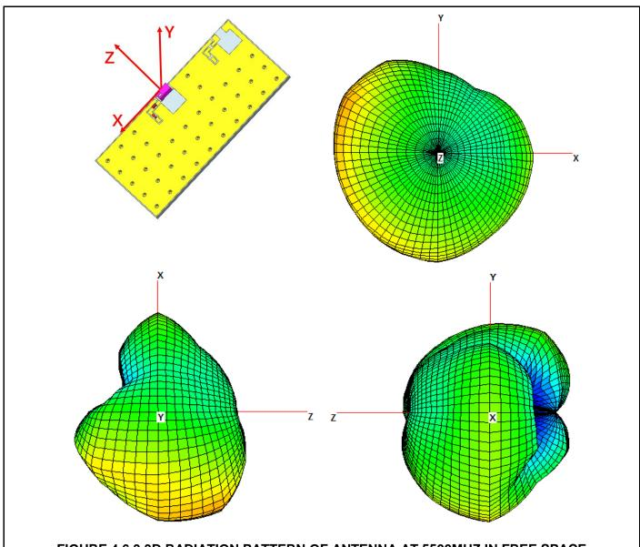
FIGURE 4.6.3 3D RADIATION PATTERN OF ANTENNA AT 5500MHZ IN FREE SPACE FOR CONFIGURE 2
