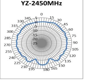
FIGURE 4.5.2 2D RADIATION PATTERN OF ANTENNA AT 2.4GHZ IN FREE SPACE FOR CONFIGURE 2
