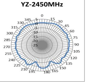
FIGURE 4.5.1 2D RADIATION PATTERN OF ANTENNA AT 2.4GHZ IN FREE SPACE FOR CONFIGURE 1
