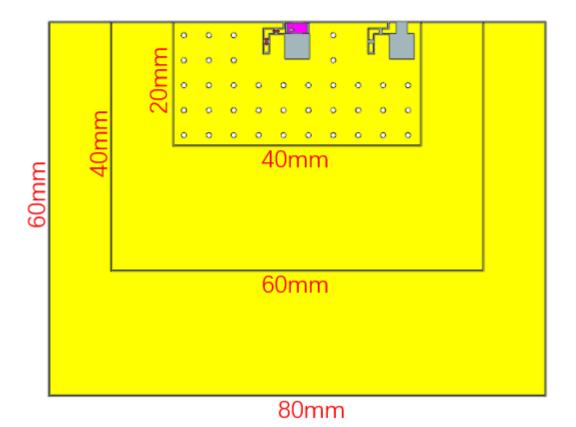
FIGURE 7.4 ANTENNA WITH DIFFERENT PLANE GROUNDS (USING CONFIG1 FOR ILLUSTRATION)
