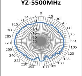
FIGURE 4.5.3 2D RADIATION PATTERN OF ANTENNA AT 5.5GHZ IN FREE SPACE FOR CONFIGURE 2
