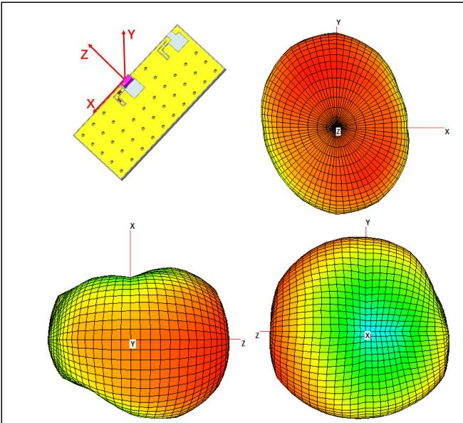
FIGURE 4.6.2 3D RADIATION PATTERN OF ANTENNA AT 2450MHZ IN FREE SPACE FOR CONFIGURE 2
