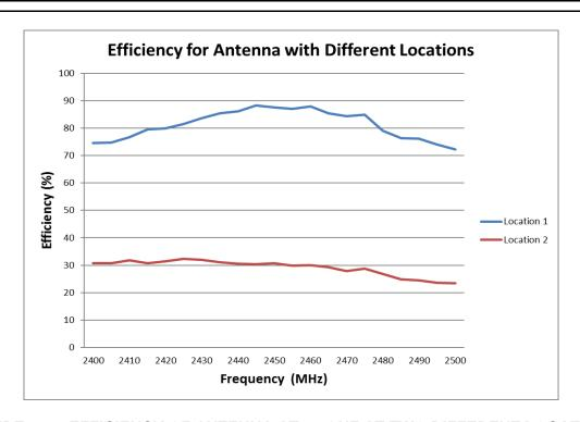
FIGURE 7.3.4 EFFICIENCY OF ANTENNA AT 2.4GHZ AT TWO DIFFERENT LOCATIONS FOR CONFIGURE 1
