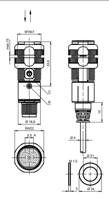
A Optical axis B Indicator diode
