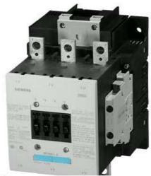
CONTACTOR, 90KW/400V/AC-3, AC(40...60HZ)/DC OPERATION UC 240...277V AUXIL. CONTACTS 2NO+2NC 3-POLE, SIZE S6 BAR CONNECTIONS CONVENT. OPERATING MECHANISM SCREW TERMINAL
