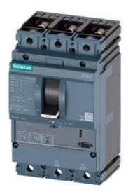
CIRCUIT BREAKER 3VA2 IEC FRAME 160 BREAKING CAPACITY CLASS M ICU=55KA @ 415 V 3POLE, LINE PROTECTION ETU320, LI, IN=100A OVERLOAD PROTECTION IR=40A ...100A SHORT CIRCUIT PROTECTION II=12 X IN BUSBAR CONNECTION
