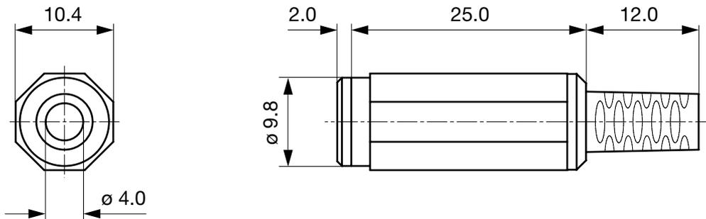
Cable diameter max. 4.0 mm
