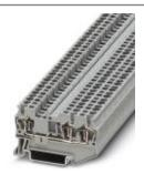
Feed-through terminal block, Connection method: Spring-cage connection, Cross section: 0.08 mm² - 4 mm², AWG: 28 - 12, Width: 5.2 mm, Color: gray, Mounting type: NS 35/7,5, NS 35/15
