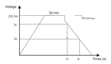
I - Discharge Current [mA], 4 \* C \* VR VR - Rated Voltage
