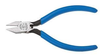
Sharp pointed nose for precise tip cutting and trimming printed circuit boards. Spring-loaded for self-opening action. Short jaws and beveled cutting edges permit close cutting of wire. Induction-hardened cutting knives for long life. Hot-riveted joint ensures smooth action and no handle wobble. Plastic-dipped handles for comfort and ease of identification. Custom, US-made tool steel.
