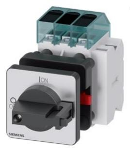
Switch disconnector 3LD3, main switch 3-polig, lu 32A operational switch at AC-23 A at 400 V 11,5 kW front mounted Base mounting with center-hole 22,5 mm knob-operated mechanism black 48 x 48 mm with auxiliary 1NO+1NC
