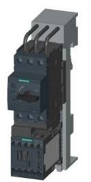
LOAD FEEDER FUSELESS DIRECT START, AC 400V, SZ S00 1.8. . .2.5A, AC 230V SCREW CONNECTION FOR BUSBAR SYSTEMS 60MM TYPE OF COORDINATION 2, IQ = 150KA (ALSO FULFILLS TYPE OF COORDINATION 1) 1NO (CONTACTOR)
