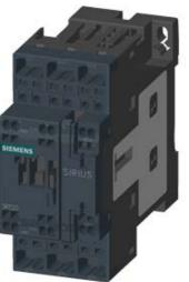
CONTACTOR, AC-3, 5.5KW/400V, 1NO+1NC, AC(50-60HZ)/DC ACTUAT. AC/DC 21...28V, 3-POLE, SZ S0 SPRING-LOADED TERMINAL
