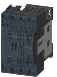
4NO CONTACTOR, AC1: 35A AC 24V 50HZ 4-POLE, 4NO, SZ: S0, SPRING-LOADED TERMINAL 1NO+1NC INTEGR.
