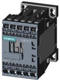
2NO+2NC CONTACTOR, AC3: 4KW DC 24V 4-POLE, 2NO+2NC, SZ: S00, SPRING-LOADED TERMINAL
