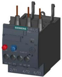
OVERLOAD RELAY 5.5...8.0 A FOR MOTOR PROTECTION SZ S0, CLASS 10, F. MOUNTING ONTO CONTACTOR MAIN CIRCUIT: SCREW TERMINAL AUX. CIRCUIT: SCREW TERMINAL MANUAL-AUTOMATIC-RESET
