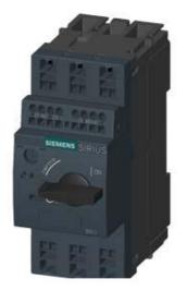
SPECIAL TYPE CIRCUIT BREAKER SIZE S00, FOR MOTOR PROTECTION, CLASS 10, A-RELEASE 2.8...4A, SHORT-CIRCUIT RELEASE 52A, SPRING-LOADED TERMINAL, STANDARD SWITCHING CAPACITY W. TRANSVERSE AUXILIARY SWITCH 1NO+1NC AMBIENT TEMPERATURE -50 DEGREES C 500 SWITCHING CYCLES
