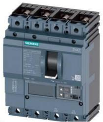
CIRCUIT BREAKER 3VA2 IEC FRAME 100 BREAKING CAPACITY CLASS L ICU=150KA @ 415 V 4POLE, LINE PROTECTION ETU860, LSIG, IN=63A OVERLOAD PROTECTION IR=25A ...63A SHORT CIRCUIT PROTECTION ISD=0,6..10X IN, II=1,5..12X IN NEUTRAL PROTECTION ADJUSTABLE (OFF, UPTO 160%) GROUNDFAULT, SWITCHABLE IG=0,2... 1 X IN, TG=0,050,8MS BUSBAR CONNECTION
