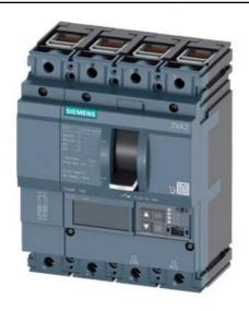
CIRCUIT BREAKER 3VA2 IEC FRAME 160 BREAKING CAPACITY CLASS M ICU=55KA @ 415 V 4POLE, LINE PROTECTION ETU560, LSIG, IN=25A OVERLOAD PROTECTION IR=10A ...25A SHORT CIRCUIT PROTECTION ISD=0,6..10X IN, II=1,5..12X IN NEUTRAL PROTECTION ADJUSTABLE (OFF, UPTO 160%) GROUNDFAULT, SWITCHABLE IG=0,2... 1 X IN, TG=0,050,8MS CABLE CONNECTION
