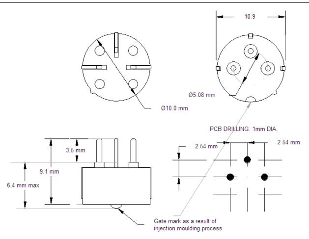
INSULATOR: 30% GLASS FILLED POLYESTER RATED UL94V-0 CONTACT: NICKEL GOLD PLATED PHOSPHOR BRONZE.
