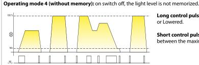
Long control pulse: The light level is progressively raised or Lowered.
