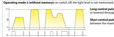
Long control pulse: The light level is progressively raised or lowered through a maximum of 10 incremental steps.
