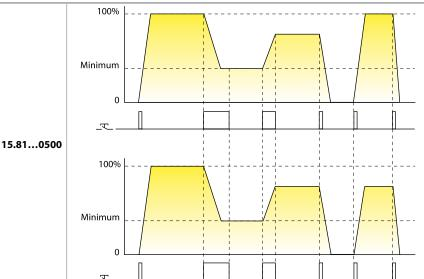
**Operating mode without memory:** at switch-off, the light level is not memorized.
