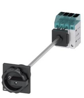
Load disconnector 3LD3, lu 63 A Main switch 3-pole + N Rated operating capacity at AC-23 A at 400V 22.0 kW floor mounting Basic switch with door coupling Central hole mounting 22.5mm Rotating drive black 66 x 66 mm
