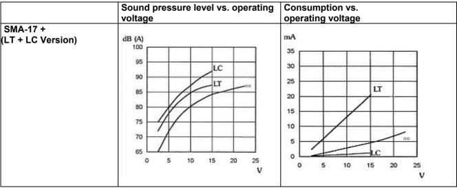
All measurements are made at 30 cm in free air at 21°C.
