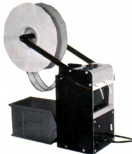
PM-1 with Motor Drive MD-1. (Showing alternative bin mounting position, large bin is not supplied)
