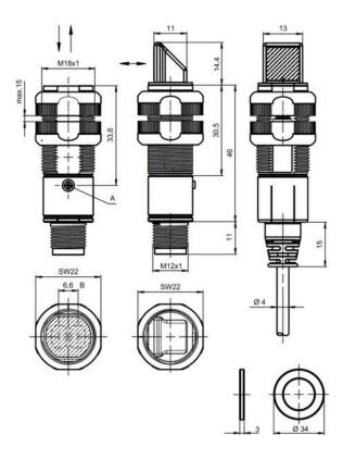
B Optical axis A Indicator diode
