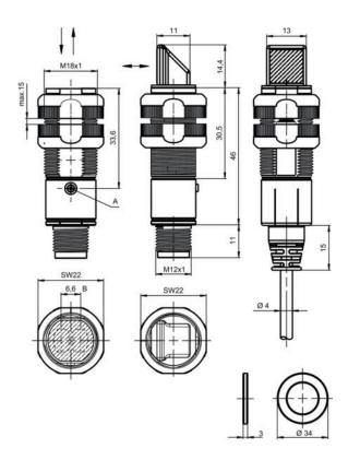
B Optical axis A Indicator diode
