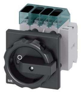
Switch disconnector 3LD3, main switch 3-polig + N, lu 63A operational switch at AC-23 A at 400 V 22,0 kW front mounted Base mounting with center-hole 22,5 mm knob-operated mechanism black  $66\ x66$  mm with auxiliary 1NO+1NC
