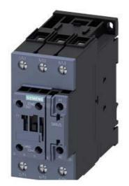
CONTACTOR,AC3:22KW/400V, 1NO+1NC, 48V AC 50/60HZ, 3-POLE, SIZE S2, SCREW TERMINAL
