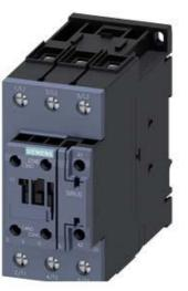
CONTACTOR,AC3:22KW/400V, 1NO+1NC, 20-33V AC/DC, WITH VARISTOR, 3-POLE, SIZE S2, SCREW TERMINAL
