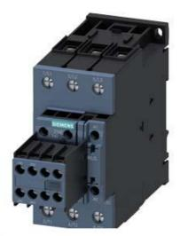
CONTACTOR,AC3:37KW/400V, 2NO+2NC, 175-280V AC/DC, WITH VARISTOR, 3-POLE, SIZE S2, SCREW TERMINAL
