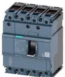
CIRCUIT BREAKER 3VA1 IEC FRAME 100 BREAKING CAPACITY CLASS N ICU=25KA @ 415 V 4-POLE, LINE PROTECTION TM210, FTFM, IN=16A OVERLOAD PROTECTION IR=16A FIXED SHORT CIRCUIT PROTECTION II=10 X IN NEUTRAL UNPROTECTED CABLE CONNECTION
