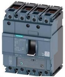
CIRCUIT BREAKER 3VA1 IEC FRAME 160 BREAKING CAPACITY CLASS H ICU=70KA @ 415 V 4-POLE, LINE PROTECTION TM240, ATAM, IN=80A OVERLOAD PROTECTION IR=56A ...80A SHORT CIRCUIT PROTECTION II=5...10 X IN NEUTRAL UNPROTECTED CABLE CONNECTION
