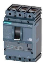
CIRCUIT BREAKER 3VA2 IEC FRAME 100 BREAKING CAPACITY CLASS L ICU=150KA @ 415 V 3POLE, LINE PROTECTION ETU330, LIG, IN=100A OVERLOAD PROTECTION IR=40A ...100A SHORT CIRCUIT PROTECTION II=1,5...12 X IN GROUNDFAULTPROTECTION IG=0,2... 1 X IN, TG=0,1/0,3MS CABLE CONNECTION
